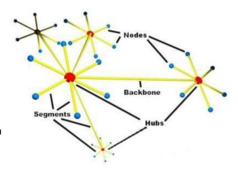
Nodes in particular areas are connected to hubs or switches (creating stars) nodes in particular areas are connected to hubs or switches (creating stars). Hubs or switches are connected together along the network backbone (like a bus network).
